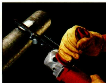
Strap polishing using contact arm 48-08-0290.
