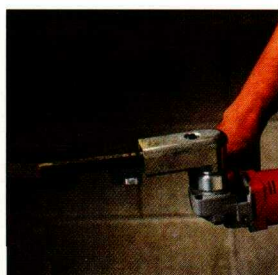
Grind and deburr ends of metal stock.
